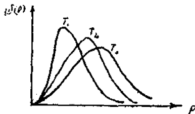
5-chizma. Temperatura qiymati-ning o'zgarishiga qarab Maksvell taqsimoti grafikasining o'zgarishi T_1 < T_2 < T_3
