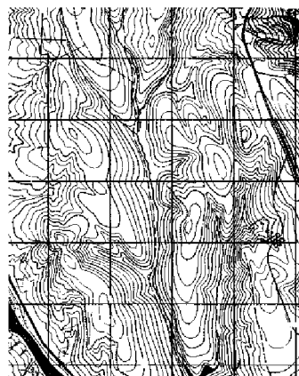
56-rasm. Relyefni gipsometrik (a) va gorizontallar (b) bilan ifodalash.
