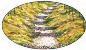
2 stone walls across waterways, they prevent hillsides from erosion during heavy rains
